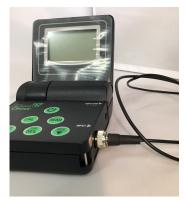
To connect the probe to the meter, orient the BNC connector to the port and insert it. Then give it 90 degree twist clockwise.
