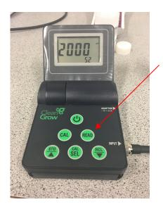
Before testing samples, make sure the previous steps have been completed. To begin testing, insert the probe into the sample. Following the prior instructions on inserting and removing the probe from solutions. Then, press the 'Read' button( see red arrow).
