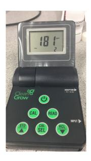
Once the reading is complete, the results will be displayed on screen in ppm.
