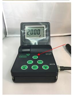
Once the probe has soaked in the conditioning solution, you can turn the probe on using the power button (see red arrow). Once the probe is turned on, there is a live mV reading displayed.
