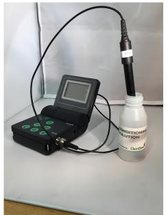
When you remove the probe from each solution, shake of thoroughly to get the excess solution out from inside the probe, and dry of the outside. When inserting the probe into a solution, shake vigorously to remove any air bubbles.
