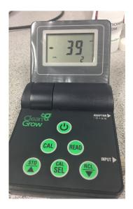
To begin calibration, select your calibration type. This is done by pressing the 'Cal Sel' button. The calibration type is displayed on screen (see red arrow).
