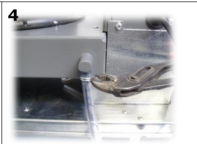
Place the collar as close to the pipe as possible
