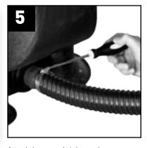
Attach hose and tighten clamp.
