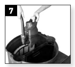
Lower pump into Skimmerfilter™ chamber
