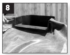
Next, install the remaining screws halfway. Tighten all screws evenly **by hand**, until flush with the faceplate.
