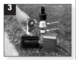
Put teflon tape onto pump connector threaded fitting and adapter. Assemble in the order shown.
