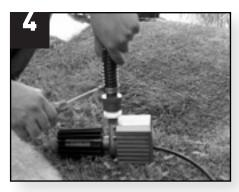
Press hose onto pump adapter and secure with hose clamp provided.
