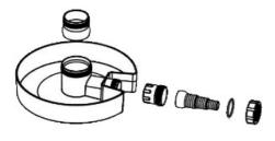
2. NEXT ASSEMBLE CENTER PIPE TOGETHER AND PLACE DEBRIS BASKET AND FLOATING SLEEVE INTO POSITION.
