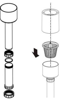
3. NOW ASSEMBLE CENTER PIPE ONTO THE BASE OF SKIMMER.
