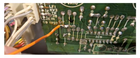
Now connect the 2 pin connector to the FILTER connector on the midi board as shown in image.
