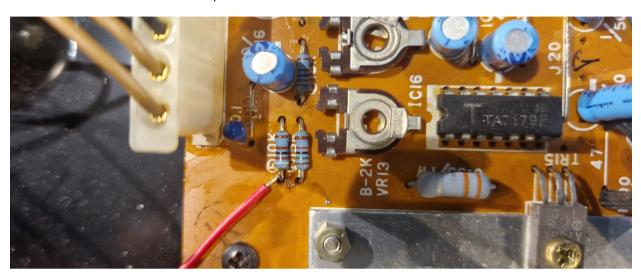
Locate the solder point shown in image. Solder the **blue wire** to this point.
