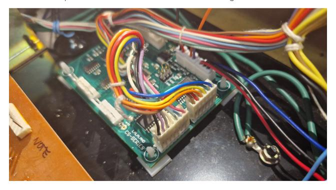
Now connect the provided 7 Pin cable to the Keyboard PCB as shown in image.
