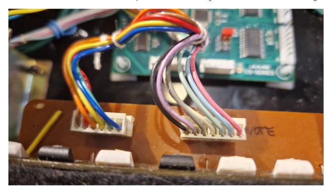
Connect the 7 pin cable to the midi board as shown in image.
