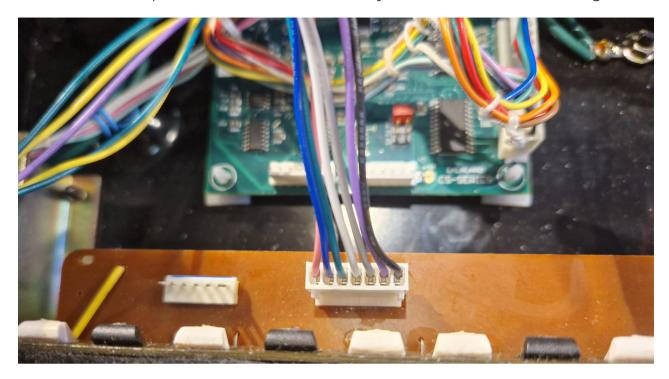
Connect the provided 6 pin cable to the Keyboard PCB as shown in image.
