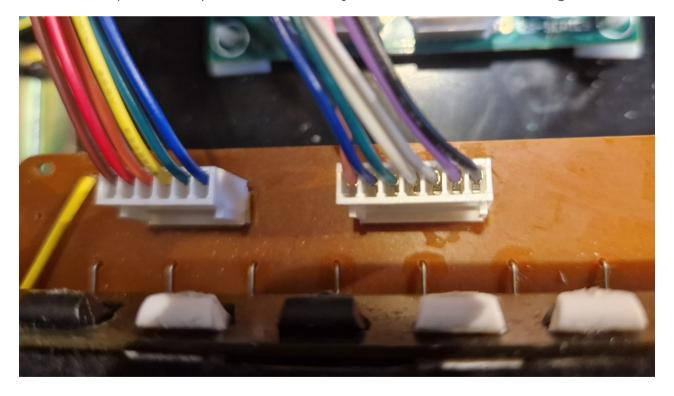
Connect the 6 and 7 pin cables to the MIDI board as shown in image.
