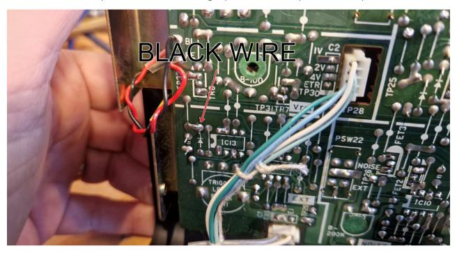
**Use the provided white and black cable.** (White is not used in the CS5) Solder the Black wire to this point using the provided 1k resistor.
