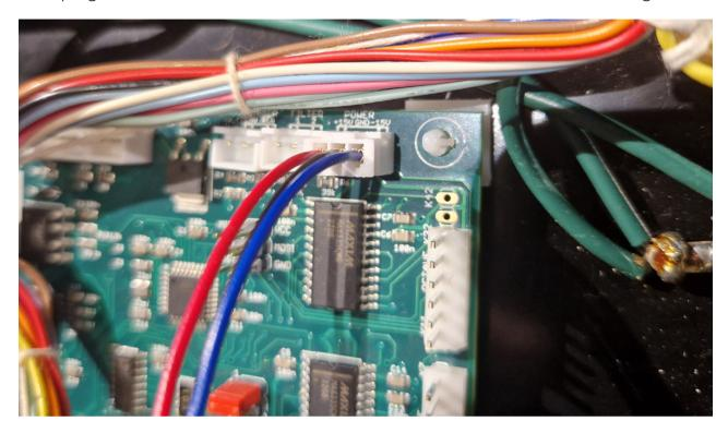
Locate and disconnect the 6 and 7 pin cables on the keyboard PCB as shown in image.
