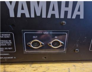
Place the midi kit as shown in image below. Fasten the board using the plastic standoffs or drill a hole and mount using screws.
