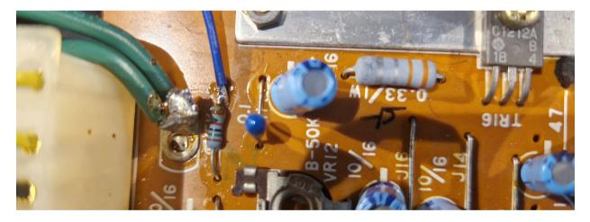
Locate the solder point shown in image. Solder the **black wire** to this point.
