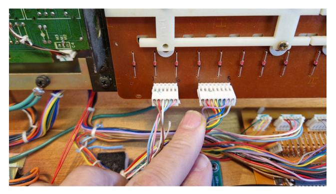
Connect the 6 and 8 pin cables to the midi board.
