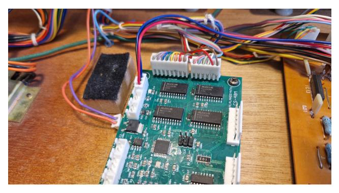
Connect the provided 6 pin cable to the keyboard PCB
