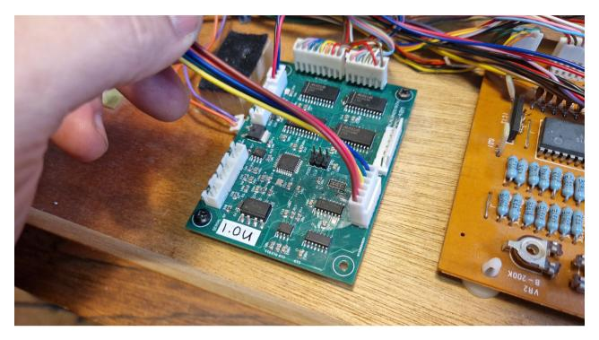
Connect the provided 8 pin cable to the Keyboard PCB.
