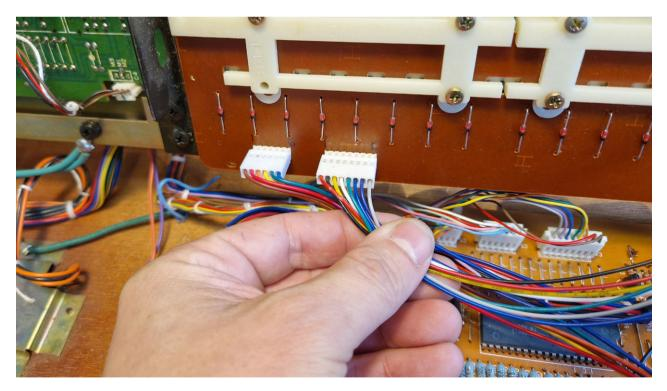
Connect the 8 pin cable to the MIDI board.
