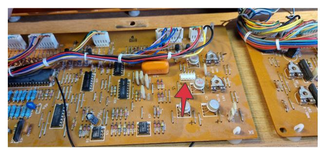
Using the 5 Wire (Red, Black, Blue) power cable, insert the connector while taking care of the correct orientation.
