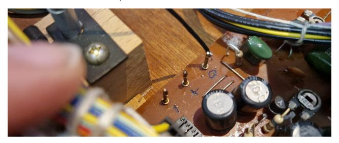
Locate the solder point shown in image. Solder the **red wire** to this point.
