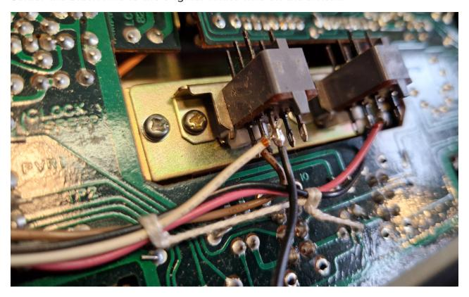
Solder the provided 10k resistor from the black wire to the GND on the pcb.
