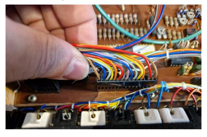
Connect the 15 pin cable you just disconnected to the provided 15 pin FEMALE cable. Match the 1 empty connector and wire colors to orient the cables in the correct way.
