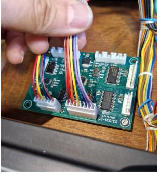
Now connect the provided 15 pin MALE cable to the SSK Board where you previously removed the original cable while making note of the one empty connector and colors. Brown and RED are on the right hand side as shown in image.
