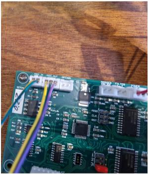
NOTE: At this point the board, MIDI in/out is operational. Filter, envelope and SEQ are optional.
