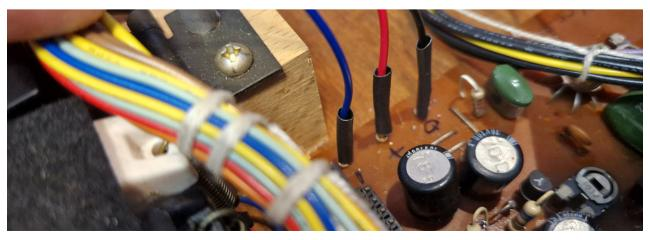
Now plug in the Power cable into Power on the MIDI Board as shown in image.
