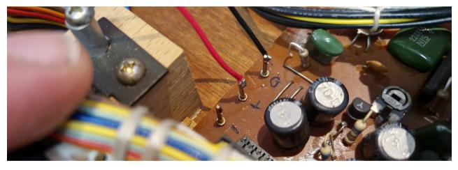
Locate the solder point shown in image. Solder the **blue wire** to this point.
