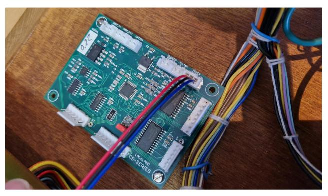
Locate and disconnect the 15 pin cable on the SSK/Key Assigner PCB as shown in image. Center board, bottom of synth.
