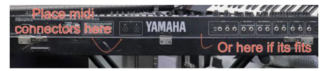
Place the midi kit as shown in image below. Fasten the board using the plastic standoffs.
