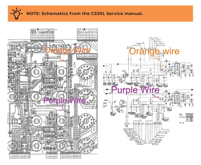
Now connect the 2 pin connector to the FILTER connector on the midi board as shown in image.
