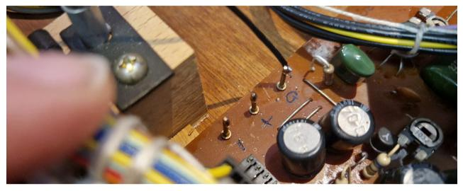
Locate the solder point shown in image. Solder the **red wire** to this point.
