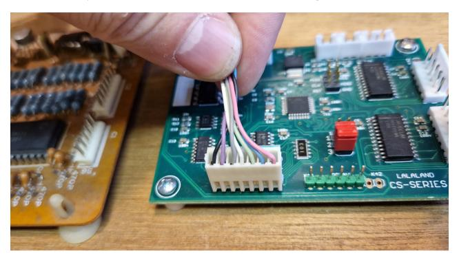
Connect the 6 pin cable to the midi board as shown in image.
