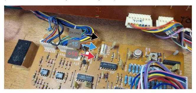
Using the 3 Wire (Red, Black, Blue) power cable, insert the connector while taking care of the correct orientation.
