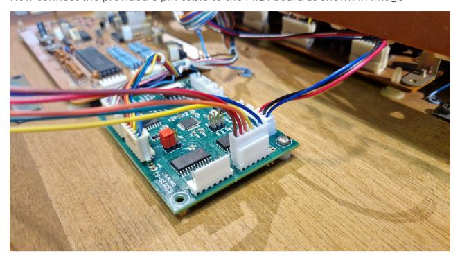
Connect the provided 7 pin cable to the MIDI board as shown in image
