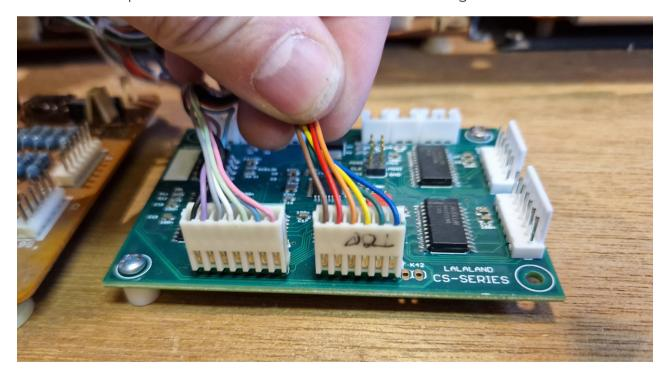
Now connect the provided 6 pin cable to the MIDI board as shown in image
