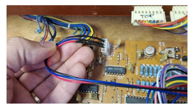
Now plug the Power cable into Power on the MIDI Board as shown in image.
