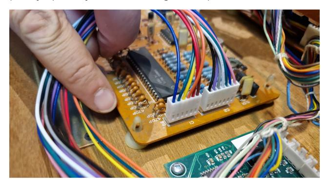
Connect the MIDI in and out cables as shown in image.
