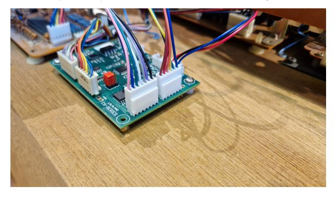
Connect the 6 and 7 pin cables to the MIDI board as shown in image. (where you previously disconnected the original cables).
