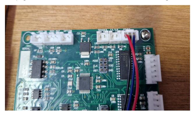
Locate and disconnect the 6 and 7 pin cables on the key assigner PCB.
