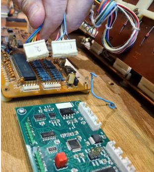
Connect the 7 pin cable to the midi board as shown in image.
