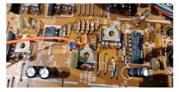
Now connect the 2 pin connector to the FILTER connector on the midi board as shown in image.
