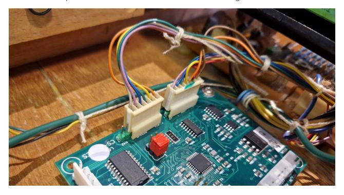
Now connect the provided 6 pin cable to the Key Assigner PCB as shown in image (where you previously diconnected the original cables).
