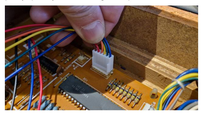
Connect the provided 7 pin cable to the Keyboard PCB as shown in image (where you previously diconnected the original cables).
