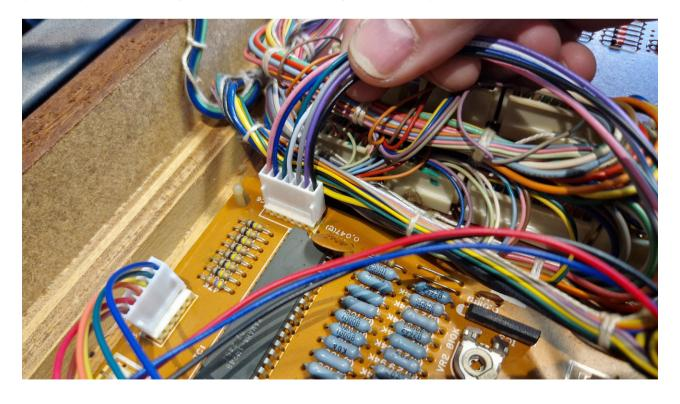
Connect the 6 and 7 pin cables to the MIDI board as shown in image.
