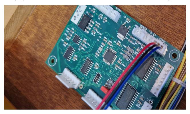
Locate and disconnect the 6 and 7 pin cables on the key assigner PCB. Upper left, bottom of the synth.
