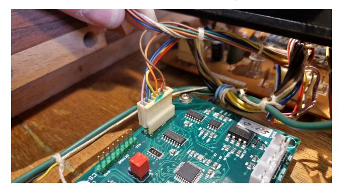
Connect the 6 pin cable to the midi board as shown in image.
