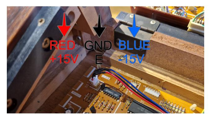
Now plug in the Power cable into Power on the MIDI Board as shown in image.C
