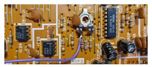
Now connect the 2 pin connector to the FILTER connector on the midi board as shown in image.
