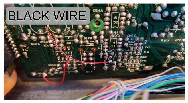
Use the provided white and black cable (white is not used). Solder the black wire to this point shown in image using the provided 1k resistor.
