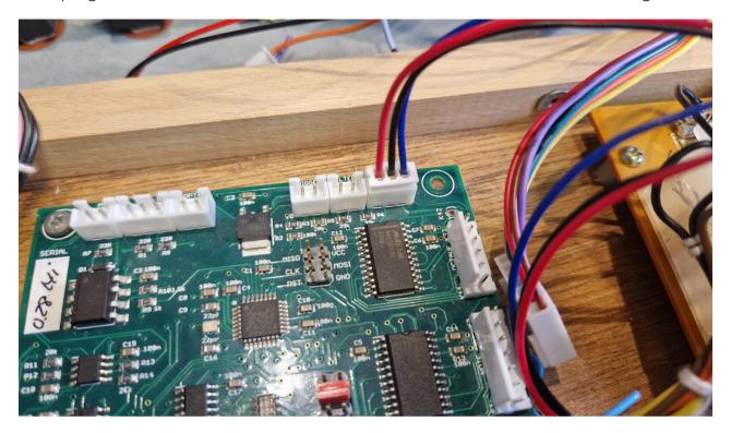
Locate and disconnect the 20 pin cable on the keyboard PCB as shown in image.
