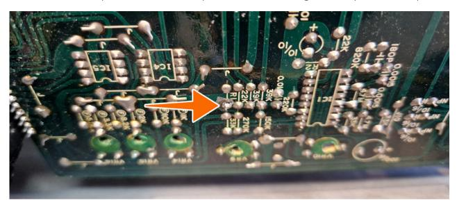
Use the provided orange and Purple cable. Solder the orange wire to this point shown in image (Purple is not used in the CS5)
