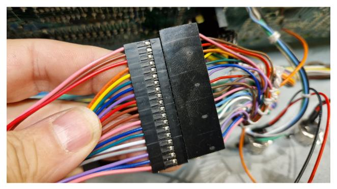
Connect the 6-7 pin cables from the previous cable to the MIDI Board.
