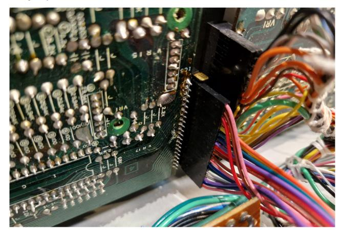
Connect the 6 and 7 pin cables from the previous cable the MIDI board as shown in image.
