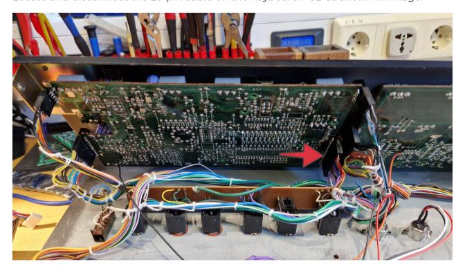
Connect the 20 pin cable to the provided female cable, match the colors and note the offset by the unused pin
