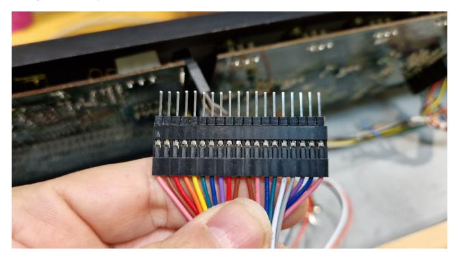
Connect the male part of the connector to the PCB (where you previously disconnected the original cable. **Note the colors and that the top pin is not used (In the synth).**
