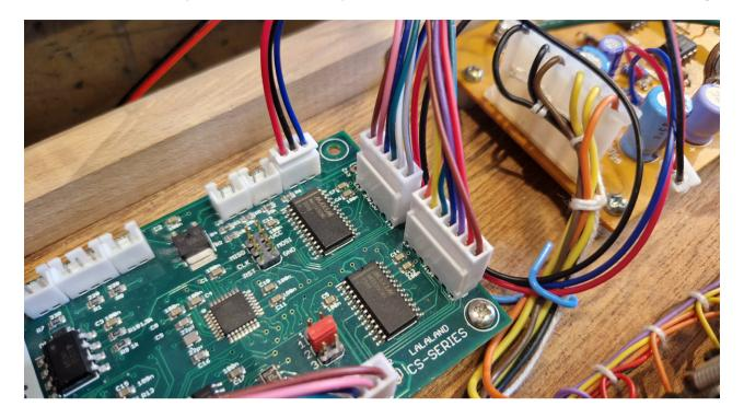
Connect the MIDI in and out cables as shown in image.
