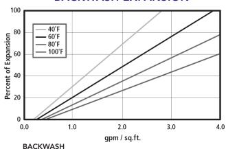
The graph above shows the expansion characteristics of Delonizer as a function of flow rate at various temperatures.
