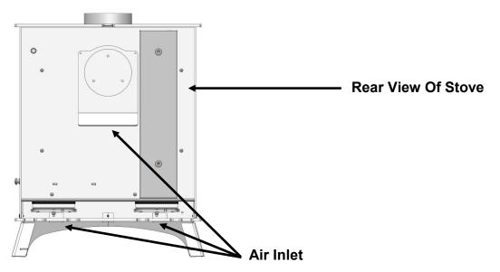
NOTE : DO NOT COVER OR PARTIALLY OBSTRUCT THE AIR INLET OPENINGS FOR THE APPLIANCE.
