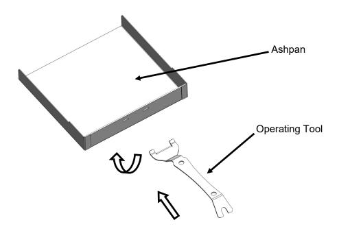
Fig. 7. Ash Pan & Operating Tool
