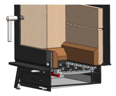
Refit the eight grate bars alternatively positioned with the heavy end in the recesses on the rocker bar and the light end on the "turrets" of the rocker bar.
