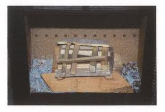
3. Move the control lever fully to the right then light the firelighters and close the door.
