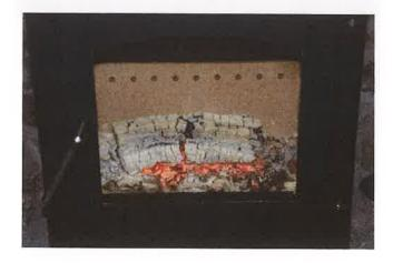
7. Move the control lever fully to the right for a few minutes to ensure a full bed of glowing charcoal, then open the door and break up the embers before placing a new log firmly on the glowing base. Close the door. The log will soon begin to flame and leave the air control open fully until the log is fully burning, the air control can then be set give the desired level of heat.
