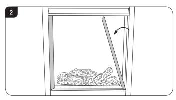
3.3 Lift out the bottom slotted trim, see Diagram 3. Note the orientation of the metal shield for reassembly.
