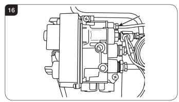
6.7 Remove the pipe and the injector drops out from the burner.
