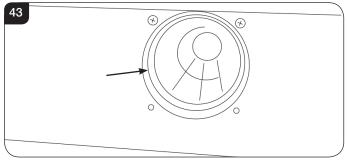
7.22 Insert 4 screws in the flanges of the flue terminal.
