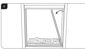
3.2 Lift out the bottom slotted trim, see Diagram 2. Note the orientation of the metal shield for reassembly.
