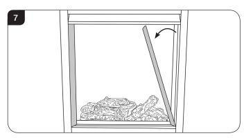
4.3 Lift out the bottom slotted trim, see Diagram 8. Note the orientation of the metal shield for reassembly.
