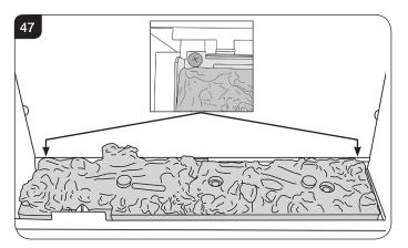
Check the pilot ensuring it is free from any debris.
