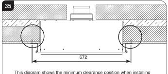
the appliance into a non-combustible wall - it is vital to ensure the batterning is wide enough to accommodate the fixings for the front.
