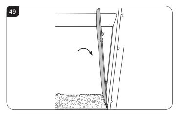
11.5 To fit the Left Hand liner insert through the front of the appliance tilting the top inwards towards the centre of the firebox before lowering into position, see Diagram 49.
