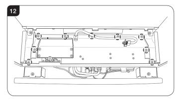
5.7 Lift the back of the control assembly and tilt forward to enable access to the controls.
