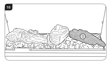
5.7 Place the right hand side of Log B on the raised stud on Log C and the left hand side on the raised section at the back left of the burner tray, see Diagrams 13 & 17.
