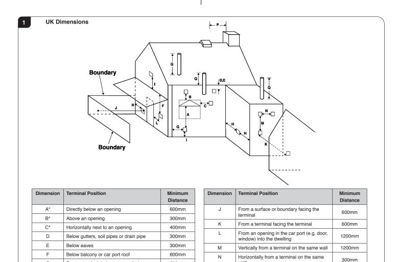
\* In addition, the terminal should not be nearer than 300mm to an opening in the building fabric formed for the purpose of accommodating a built-in element such as a window frame
