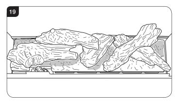
NOTE: ENSURE THAT THE LOGS ARE POSITIONED AS ABOVE. ONLY USE THE CORRECT AMOUNT OF LOGS AS SPECIFIED IN THE DIAGRAMS.
