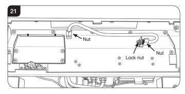
The injector can now be replaced.
