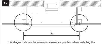
appliance into studwork - it is vital to ensure the batterning is wide enough to accommodate the fixings for the front and made from non-combustible material.
