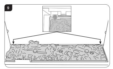
4.2 Slide the burner unit fully to the left and lift from the front. Carefully remove through the front of the appliance. Place carefully to one side. **Take care not to damage the raised area on the burner unit and the pilot unit.**
