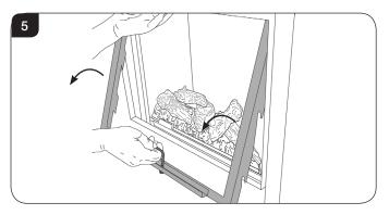
2.7 Remove the logs and Embaglow and place on a dry, clean surface.
