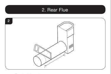
Terminal dimensions: 395 x 200 x 200 mm (H x W x D) Guard supplied Cut to length as required on site.
