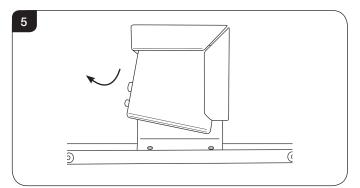
3.6 Remove the cover by sliding off in the direction of the arrow as shown in Diagram 6.
