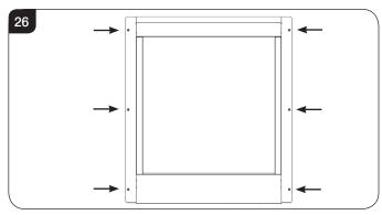
5c.10 Site the appliance, with bracket attached, into the opening. Secure into the studwork through the fixing holes in the bracket, see Diagram 27.
