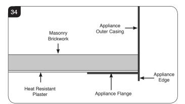
6b.6 The subframe for the decorative front can now be fitted by following the instructions supplied with the Front. NOTE: THE SUBFRAME MUST SIT FLUSH TO THE WALL LEVEL WITH THE APPLIANCE FLANGE.
