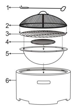
**STEP 1-** Place the MGO stand (6) on a permanent flat, level, heat resistant, non flammable surface away from flammable items.
