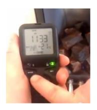
To adjust high and low whilst holding the handset and green light on press + & - to adjust for the preferred heat setting. To Stop the stove, hold handset to unlock the buttons and then press the power button. The flame stops almost immediately.
