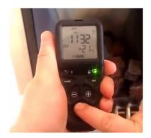
Press and hold in the power symbol button and release immediately as soon as the word pilot appears at the bottom left of the display (After about 1-2 seconds). The fire will then light onto MAX burner setting. (Note: releasing the power button too soon or holding too long
