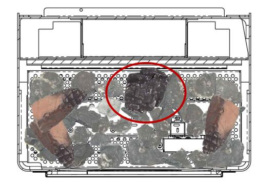
Position Log 4 as shown above, centrally at the rear of the burner.
