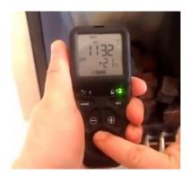
Press and hold in the power symbol button and release immediately when the word pilot appears at the bottom left of the display (After about 1-2 seconds).
