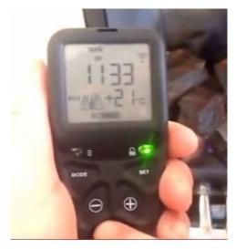
To STOP the fire, hold handset to unlock the buttons and then press the power button. The fire will stop without delay. Wait for the word OFF to appear on the display (LH Side) before trying to start again. Note:
