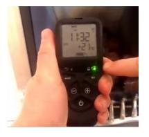
Hold the handset as shown, wrapping your hand around the handset touching both sides, and the green unlock light will illuminate allowing the buttons to work. (If the green light is not lit, the buttons will not operate).
