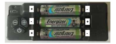
The remote display handset also has batteries as shown below. Again, remove the rear cover and replace the batteries (2 No. AA/1.5V LR6), observing the correct position as shown.
