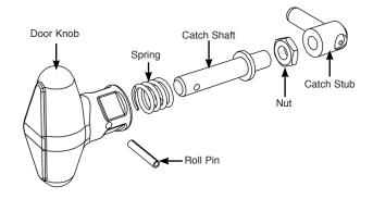
Check the door catch operation and tightness of the lock nut. Adjust if required.
