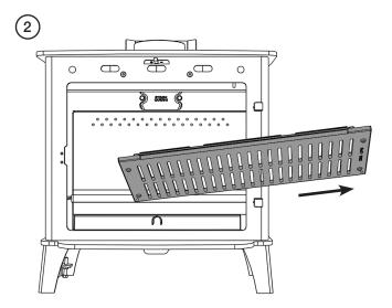
The Door Tool can be used to remove the Ash Pan.
