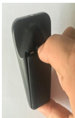
Replacing the Batteries in the Remote Controller
