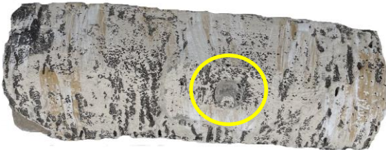
Log 1 (RH Base Log 1) – Interlocking Male Pin on top (Inside Yellow Circle)
