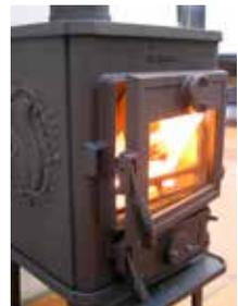
4. After 5-10 minutes the chimney draft should be established, at this point close the fire door. If all the necessary conditions are met, a nice layer of embers will start to accumulate after another 15 - 20 minutes.
