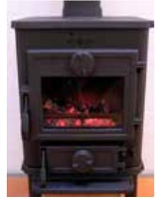
6. Place three pieces of fuel weighing roughly 0.7 kg and measuring about 30 cm in length across the embers in one layer, with spacing of roughly 1 cm between the pieces of wood.
