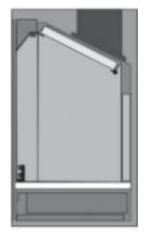
5. Fit top turbulence baffle by securing baffle plate under at front and inserting pin at rear.
