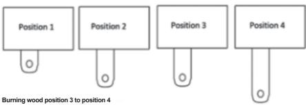
When burning coal the primary air control drops to position 3 (midpoint location) operate and regulate your stove between position 3 and 4 (fully pulled out).
