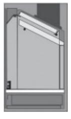
Fit baffle by placingon top of rear brick and securing with 2 steel pins into the side bricks.
