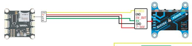
IRC Tramp telemetry pin
