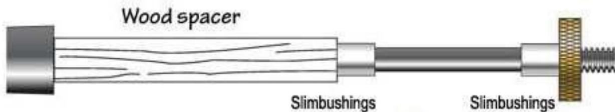
2. Advance a 60° revolving cone center into the dimpled end of the mandrel and tighten using light pressure. Do Not over tighten the tailstock or mandrel nut as this may cause the mandrel to flex resulting in off-center barrels.
