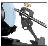
2. Set the leg angle on the tool holder to 23 degrees and lock in place. This can be done by using a protractor or by using the diagram on page 3. With a tool mounted in the Vari-Grind Jig, align the tool with the top line then adjust the leg so that the center of the leg lines up with the 23 degree line. Tighten securely.
