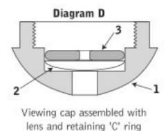
Position the viewing cap (#1) with the eyehole facing down. Drop the lens (#2) into the recess inside the cap with the convex side down, flat side up as shown. Place the lens retarding 'O' ring (#3) on top of the lens with the extending shoulder facing the lens as shown above.
