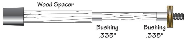
the mandrel and tighten using light pressure. **Do Not** over tighten the tailstock or mandrel nut as this may cause the mandrel to flex resulting in off-center barrels.
