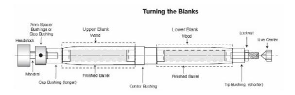
Turn your blank down to the bushings. Polish & finish blank Lay out your parts based on the diagram below
