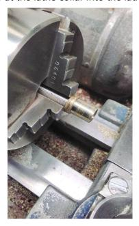
When the glue on the blank is dry, screw it into the collar.
