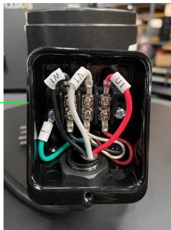
Figure 16: 110V Wiring, Junction Box
