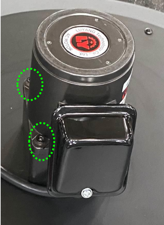
Figure 17: Autoclean Motor Mounting Bolts Figure 18: Autoclean Motor
