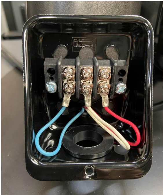
Figure 19: 220V Bottom Wiring Junction Box Figure 20: 220V Top Wiring Junction Box
