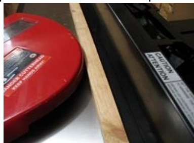
FIGURE 16: AUXILIARY FENCE IN-USE
