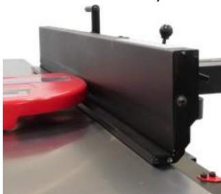
FIGURE 15: AUXILIARY FENCE LOWERED
