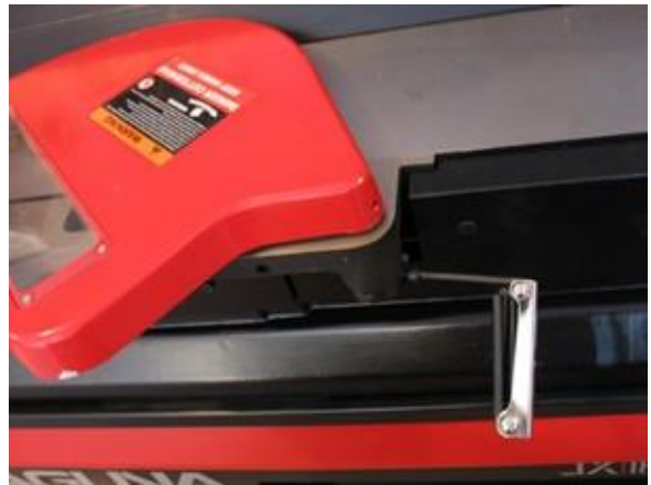
FIGURE 31: REMOVING GUARD FOR RABBETING
