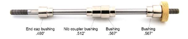
\*\*bushing measurements may vary based on pen kit using. The largest 2 are for your cap. The body has a taper toward the end cap and that will be the smallest of the 4 bushings\*\*
