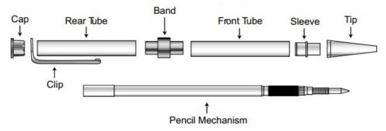
A. Press the sleeve, recessed end first into the end of the front barrel until it hits the shoulder.
