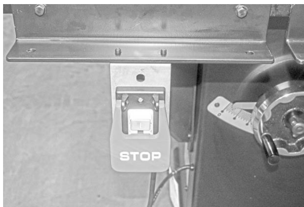
Control Switch correctly mounted. The expose bolts will fit the through holes in the fence body
