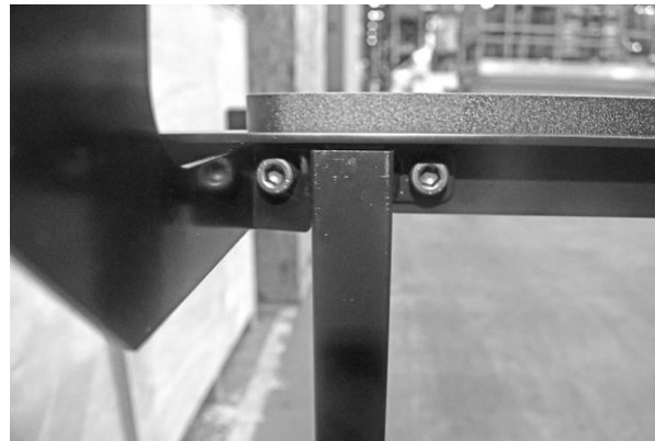
Hose support and Leg properly Installed:
