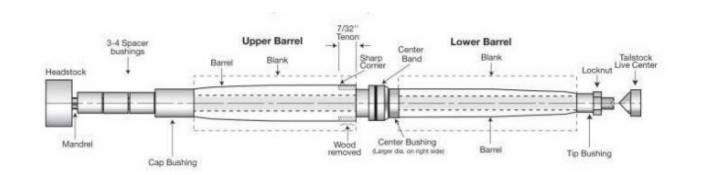
Turn your blank down to the bushings. Polish & finish blank Cutting the Tenon:
