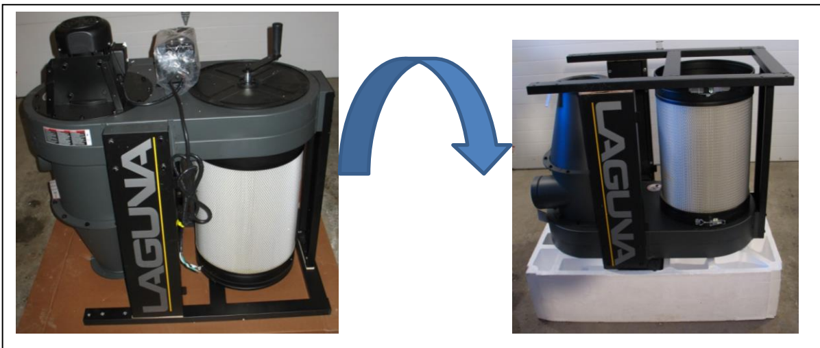
Figure 7: Placing the main component for assembly upside-down
