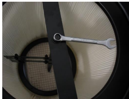
Figure 43: Removing flap pivot bolt (from underneath)
