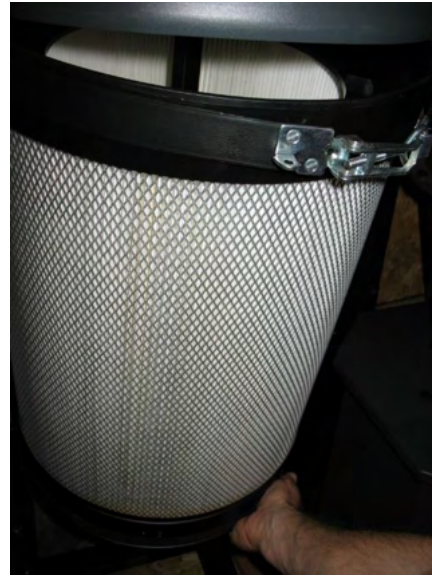
Figures 45-46: Disassembling canister for cleaning
