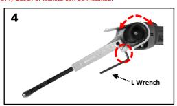
Adjust preferred angle(15-30°). and fasten the body bolt with L wrench.
