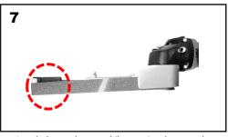
Attach the sandpaper while pressing down on the housing.
