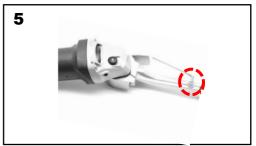
Don't tighten the fixing bolt. Just check it doesn't loosen.
