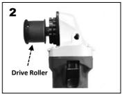
First, the roller is attached to angle grinder.
