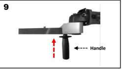
Attach the handle to the handle mounting area.
