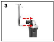
Attach the body to the grinder. (Make sure no gap in between)
