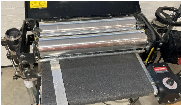
Fig. 4. Checking drum alignment (inboard side).
