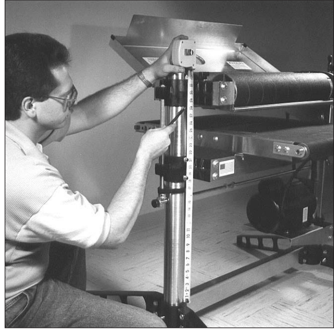
Fig. 22. Comparing drum support casting heights.
