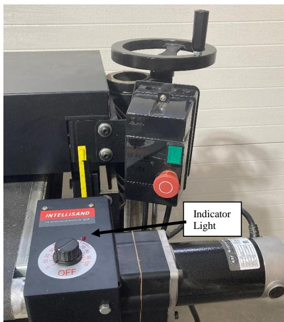
Fig. 13. Intellisand Controller and depth gauge.
