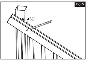
b. Trace the post onto each rail (both ends of top and bottom rails). Make four marks in total being sure to mark 1/6" shorter to allow for expansion (Fig. 5).
