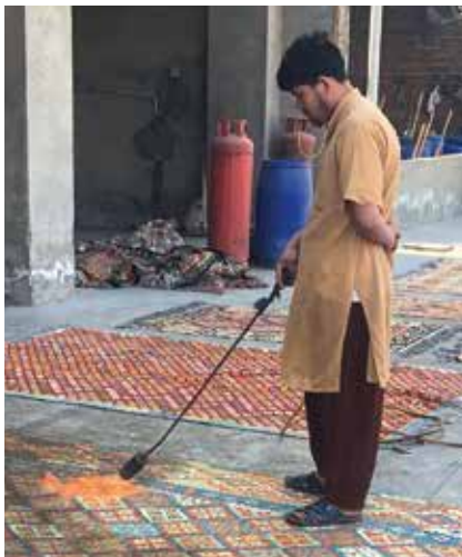
Burning the excess fluff off the Kilim.
