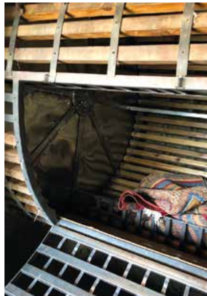
Tumbling machine, knocks out the dust.
