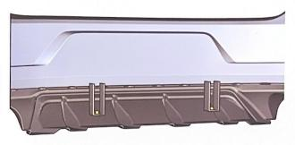
Gently push the diffuser onto the bumper to achieve the correct position. As the bumpers are often very soft in the middle and give way, make sure that you can hold against them from the inside if necessary.
