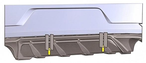
Please note that you have to remove the original plastic parts on the inside of the bumper (left & right). Drill a new hole on the underside of the bumper (marked blue) with a 7mm drill bit. As a last step you can now attach the plastic rivets through the drilled holes.
