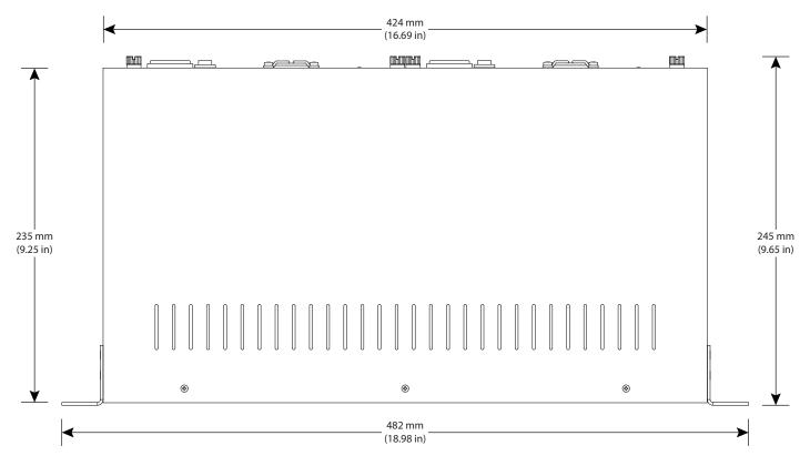
Top View with Rack Ears Installed
