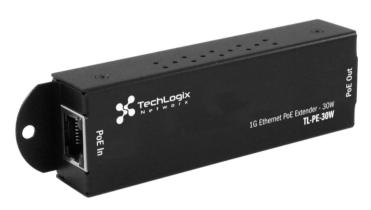
The TechLogix Networx TL-PE-30W is designed to extend connection distances from a PoE source to an output device another 100 m (328 ft.) via twisted pair cable. You can cover even longer distances by cascading these extenders on a network. The TL-PE-30W does not need any additional power supply, as it draws the power it needs from the PoE input.
