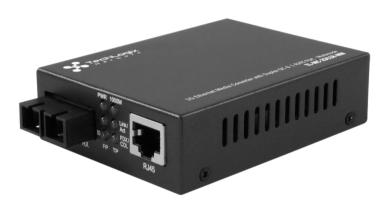
The TL-MC-2SC1R-MM features one duplex SC port (1000Base-SX) and one RJ45 twisted pair port, effectively adapting twisted pair-based devices to fiber for longer transmission distances. The TL-MC2SC1R-MM supports multimode fiber.
