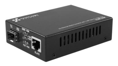
The TL-MC-1S1R features one SFP port (SFP module sold separately) and one RJ45 twisted pair port, effectively adapting twisted pair-based devices to fiber for longer transmission distances. The TL-MC-1S1R supports multimode fiber when paired with a multimode SFP module and single mode fiber when paired with a single mode SFP module.
