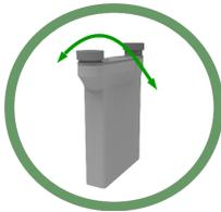
*Always invert the tank along the "long" side of the tank. (The two caps should always be at approximately the same level.) Inverting on the short axis will allow liquid to flow in/out through the baffles and can cause uneven development.*
