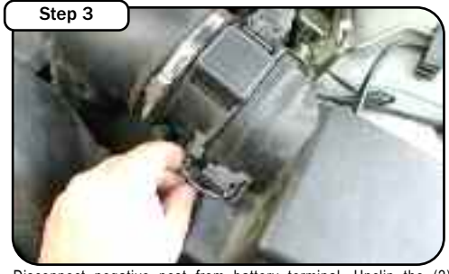
Disconnect negative post from battery terminal. Unclip the (2) spring clips that secure the MAF sensor to the air box.
