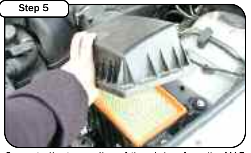
Separate the top portion of the air box from the MAF sensor by pulling straight up and out.
