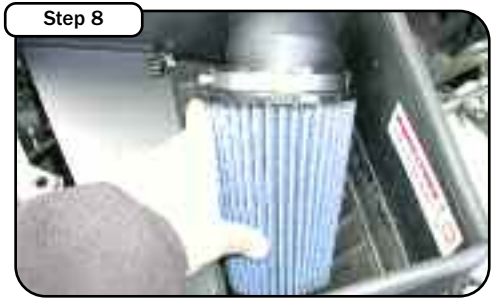
Install the pre-oiled filter in the housing and tighten down clamp. DO-NOT use any oil or grease. Install the housing trim seal around the sides of the housing.
