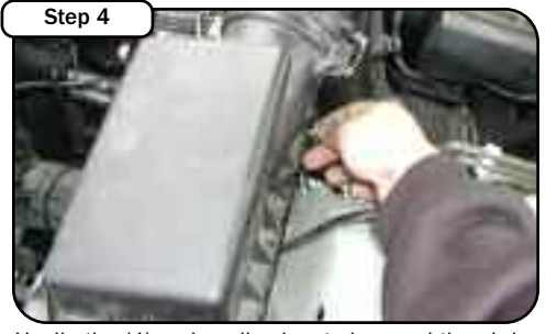
Unclip the (4) spring clips located around the air box by pulling back on the clip
