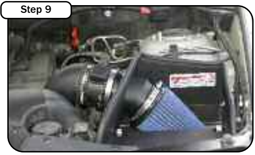
Place enclosed CARB EO sticker on or near the device on a smooth, clean surface. EO identification label is required to pass the smog inspection. Your installation is now complete. Make sure all hoses and clamps are tight and that all electrical components are secure. Check and retighten connections and filter after a few hours of operation. Close hood slowly to verify hood clearance
