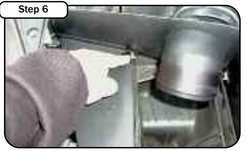
Insert the new AFE air filter housing into the lower portion of the OEM air box. Make sure the housing is placed inside the groove of the OEM box. Fasten the (4) spring clips into the new housing
