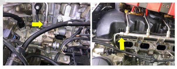
Carefully remove the connectors connecting to the HPFP and the low pressure fuel sensor
