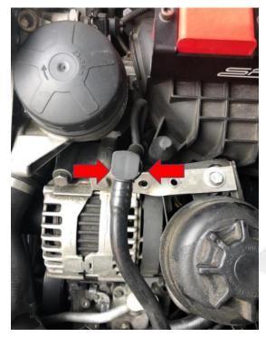
4. Remove the hard vacuum line by squeezing the tabs and pulling up.
