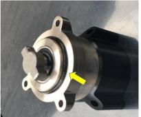
15. Optional: Remove small restrictive filter on the HPFP Inlet to be able to get full flow potential. Note: We do not recommend removing this small filter without an alternative replacement to avoid impurities from getting to injectors potentially causing leaking. We recommend our Spool 10 micron inline fuel filter kit.
