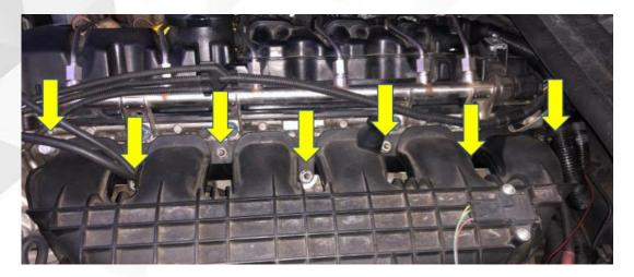
8. Carefully pull out the intake manifold making sure it doesn't get stuck on any wires.
