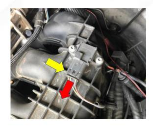
5. Remove the Vacuum line off the throttle body by pressing in the two tabs and pulling out.
