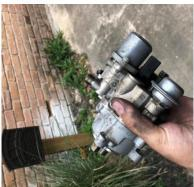
14. Remove the O-Ring around the HPFP and Install in on the helix
