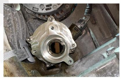
19. Install the Helix onto the new billet vacuum pump cover mounting plate. You may need to spin the Helix to help align the internal shafts.
