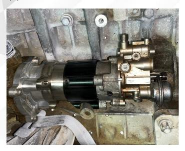
21. Secure the Spool Helix support bracket in place using the M8 x 30mm Low Head Socket Cap screw to bolt onto the block
